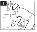
After mounting the insert tool, operate the grinder in a protected area to check that no failure occurs.
