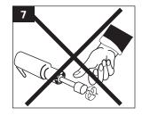
Beware of run-on. Do not touch T the tool, after turning it off, until it has stopped completely.
